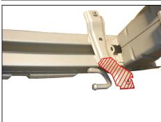
2-3 Cut off the wiring bracket.
